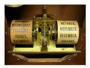
Here is a view from the back. I just turned the mechanism around for this photo. As the label below it says, no part of the calendar mechanism should ever be lubricated.
