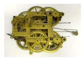
Looking at the back of the mechanism, you can see the wire, used to trip the calendar once a day.
