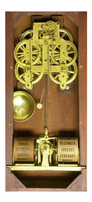
The calendar usually works well, as long as it has not been modified during any previous repairs. This calendar only required a very small adjustment to function correctly.
