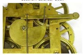
Servicing the movement is similar to other Seth Thomas clocks, such as the ST #89. The strike count lever should have a return spring, but the clearance between the count lever and the warning lever is very tight. A return spring reduces the likelihood that the detent on the count lever would jump up unexpectly, allowing the clock to strike further.
