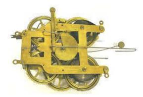
The snail allows the lever to fall. This lever and the wire hold the trip mechanism in the calendar, the weight of which moves the calendar forwards when it falls from a specified height, which is adjustable.
