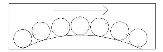
If you draw a line to trace the path of the point on the circle as it rotates along the edge of another circle, the result is called an Epicycloidal Curve.
