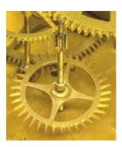
The movement must be taken apart for cleaning. The mainsprings must be removed with a mainspring winder for cleaning and inspection. Any visible damage means the mainspring must be repaired or replaced: a broken mainspring in a French clock often causes severe damage because of the fine teeth on the barrel.
