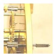
The escape wheel has very fine teeth that are very easily damaged. The pivots are very small, hard
