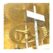
The older clocks did not have a rack and a snail in the strike mechanism. This Vincenti clock has a count wheel instead. Notice that the Vincenti clock also has a silk thread suspension, instead of a metal suspension spring.
