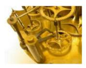
While on the subject of escapements, here is an example of the oldest design in mechanical clock escapements, the verge with crown wheel.
