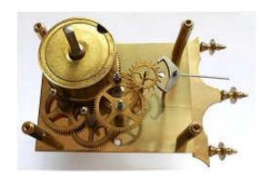
Place the back plate over the parts and insert the lower screws first. Insert the pivots into the bushing holes, one by one, working your way from the bottom up, using a pivot locator (see my page about clock tools on this website). Press down lightly on the back plate as you guide each pivot into place. If you press down hard, you could easily damage one or more of the smaller pivots.
