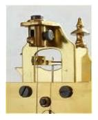
The bushings of the barrel and the first two gears should be lubricated with grease (before assembly). The bushings for the upper gears and the escapement should be lubricated with a light oil (after assembly).
