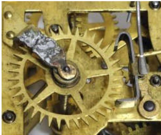
The escapement is a Strip-Pallet Recoil Escapement because the pallets are made from a strip of steel, (just like the Seth Thomas 89 above). This clock is a nice piece of American history and every collector should have one.
