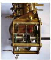
The escapement is also very precise, adjusting itself when the pendulum swings with wide amplitude. The quality is as good as you will find in any modern clock. Notice the green powder that has fallen down from the chime parts onto the gears between the plates. The grease failed when it dried.
