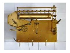
The chime mechanism uses no contrate gear, relying on three beveled gears. The parts fit together and work well without adjusting any cap screws, as you would on a Herschede. The green color is old, dry grease.
