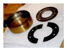
The parts from the bellows housing are deburred with a file to remove sharp corners and edges that could cut your hands.
